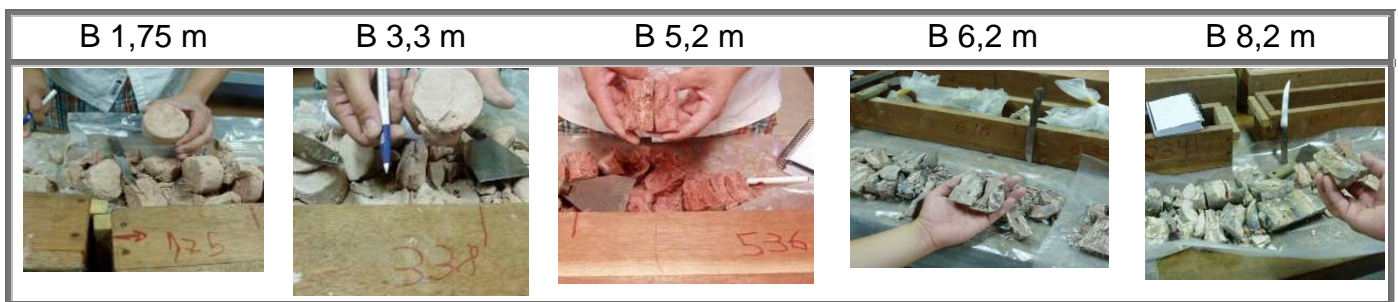
Figure 12 - Example of profile B sampling from bore holes.
