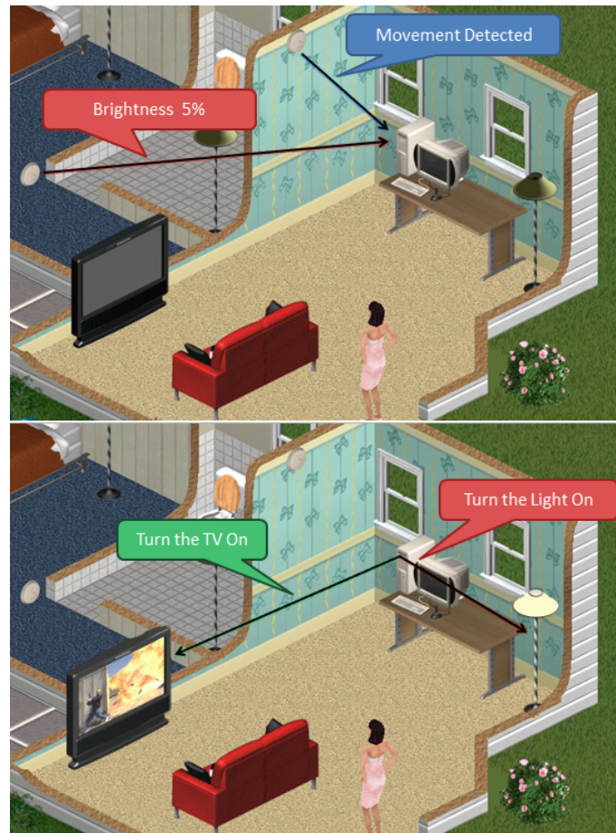
Figure 1.1: Interaction between sensor nodes and actuator nodes on a smart environment.
