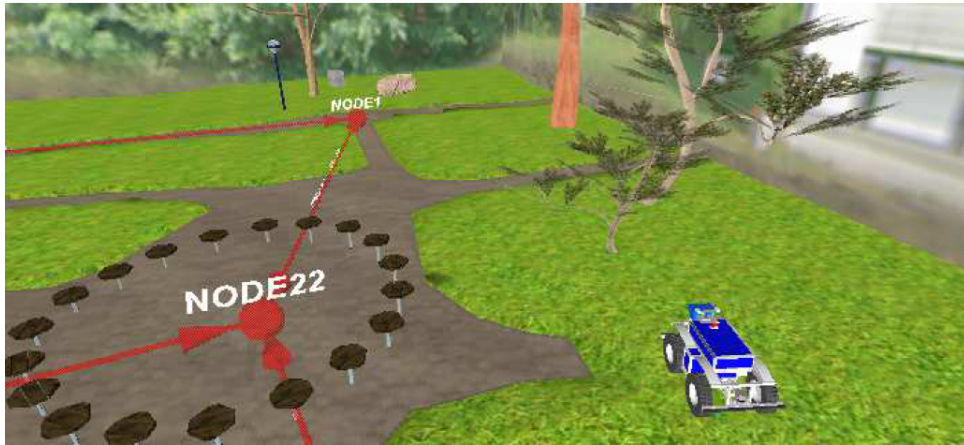
Figure 2.3: 3D-Visualization of Ravon with overlaid navigation graph (Hirth et al. 2007).
