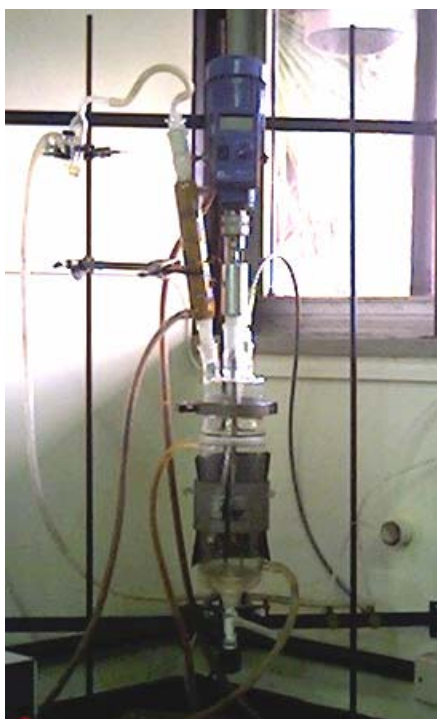
Reactor (a): Glass reactor (1 L) of continuous flow.
