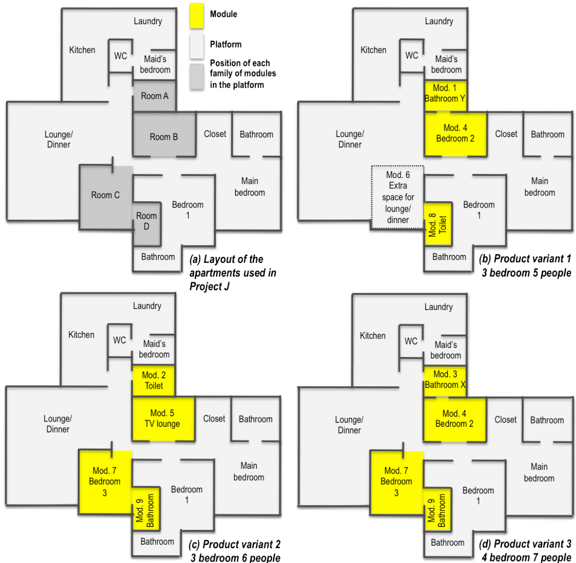
Figure 90: Schematic floor plans of the three product variants in Project J
