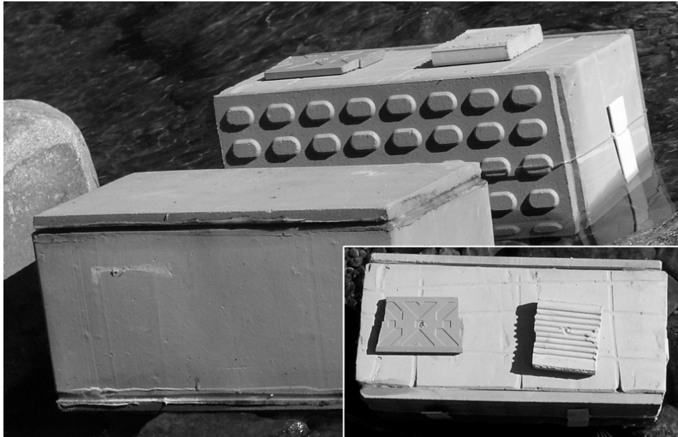
Figure 2. Bricks used as substrate in the experiment. In detail, complementary plates glued to the brick surface to increase heterogeneity.
