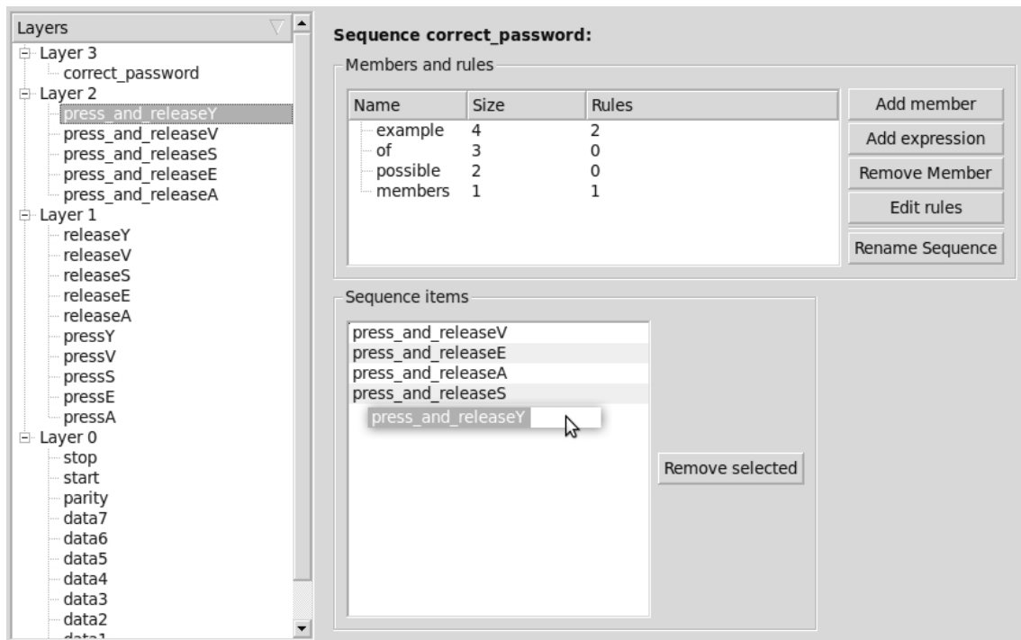
Figure 9.3: VEasy's GUI being used to build a testcase.
