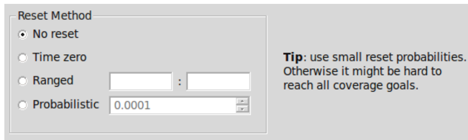
Figure 6.5: Reset methods available in VEasy's GUI.
