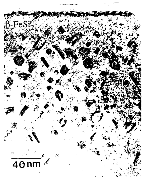
Fig. 3. Cross-sectional TEM micrograph of Fe implanted Si sample after IBIEC process and after 730°C annealing for 30 min. Note the surface layer (~ 6 nm thick) consisting of \beta\text{-FeSi}_2 precipitates. The region immediately below this layer is "dilute" in precipitates. At the deeper region there is broad distribution of \beta and \gamma precipitates.
