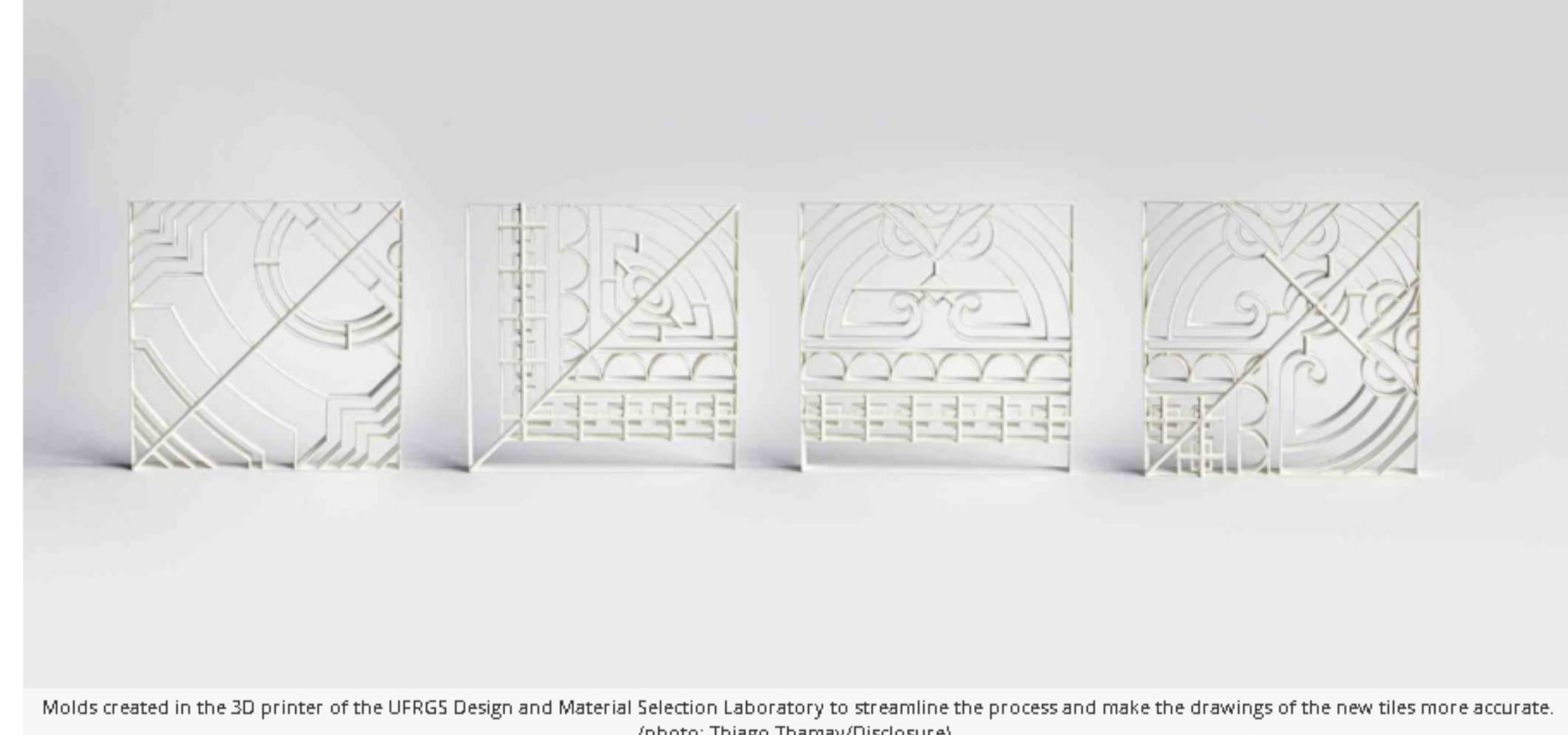
Molds created in the 3D printer of the UFRGS Design and Material Selection Laboratory to streamline the process and make the drawings of the new tiles more accurate. (photo: Thiago Thomazy/DiscoLure)
