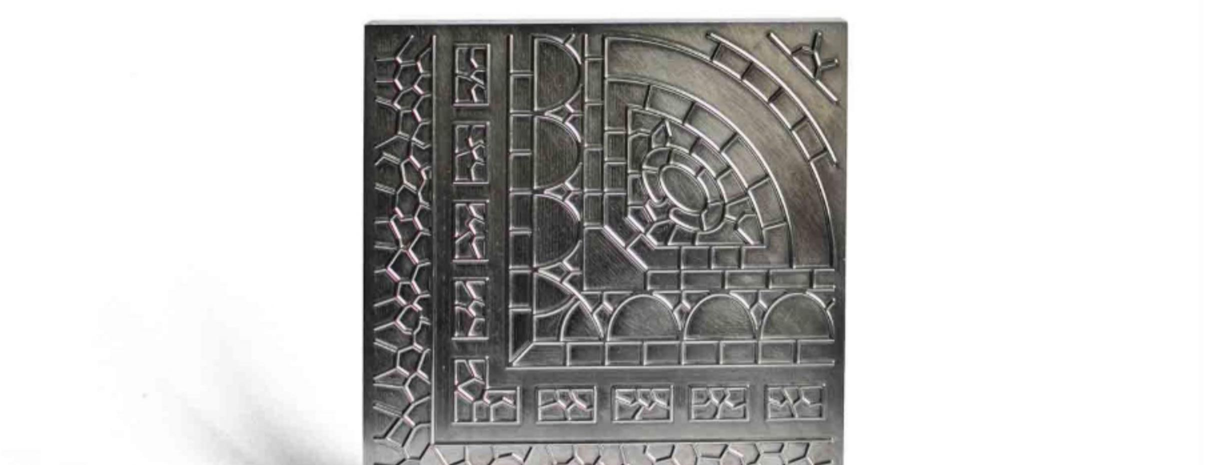
One of the steel matrices produced by the research and used to make the tiles within the standards of the Municipal Palace. (Photo: Thiago Thomazy/DiscoLure)
