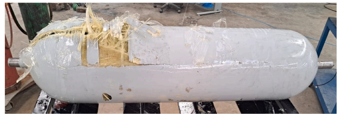
Fig. 13. Actual prototype after the burst test.
