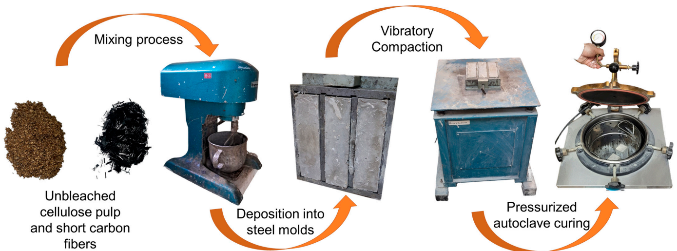
Figure 2. Composite processing and fiber-cement formulation workflow.
