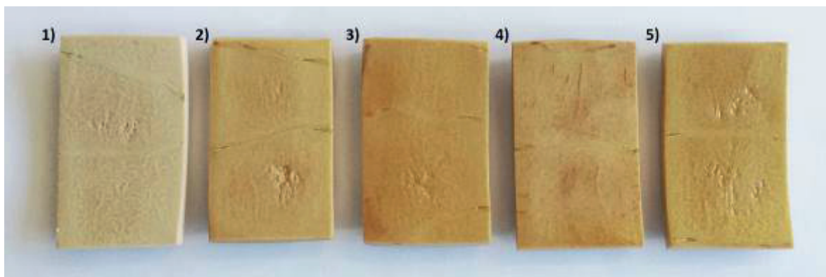
Figure 4: Samples of bottle gourd without treatment and after application of resins: 1) Sample without treatment; 2) With a layer of resin A; 3) With two layers of resin A; 4) With a layer of resin B; 5) With two layers of Resin B.
