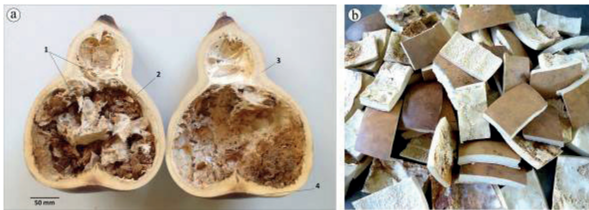
Figure 2: Samples of bottle gourd: a) fruit after the drying process in longitudinal section: (1) endocarp, (2) seeds, (3) mesocarp, (4) exocarp.; b) samples with approximate dimensions of 30 mm of width by 50 mm.
