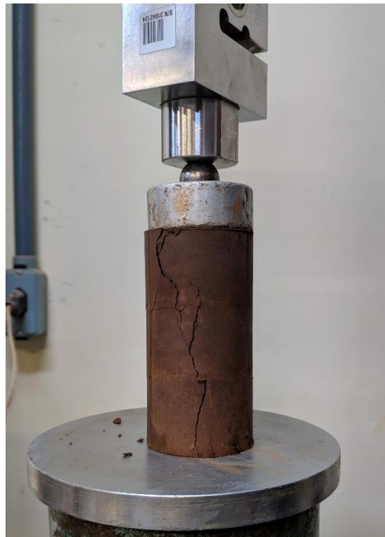
Figure 25: Unconfined compressive strength test ongoing.
