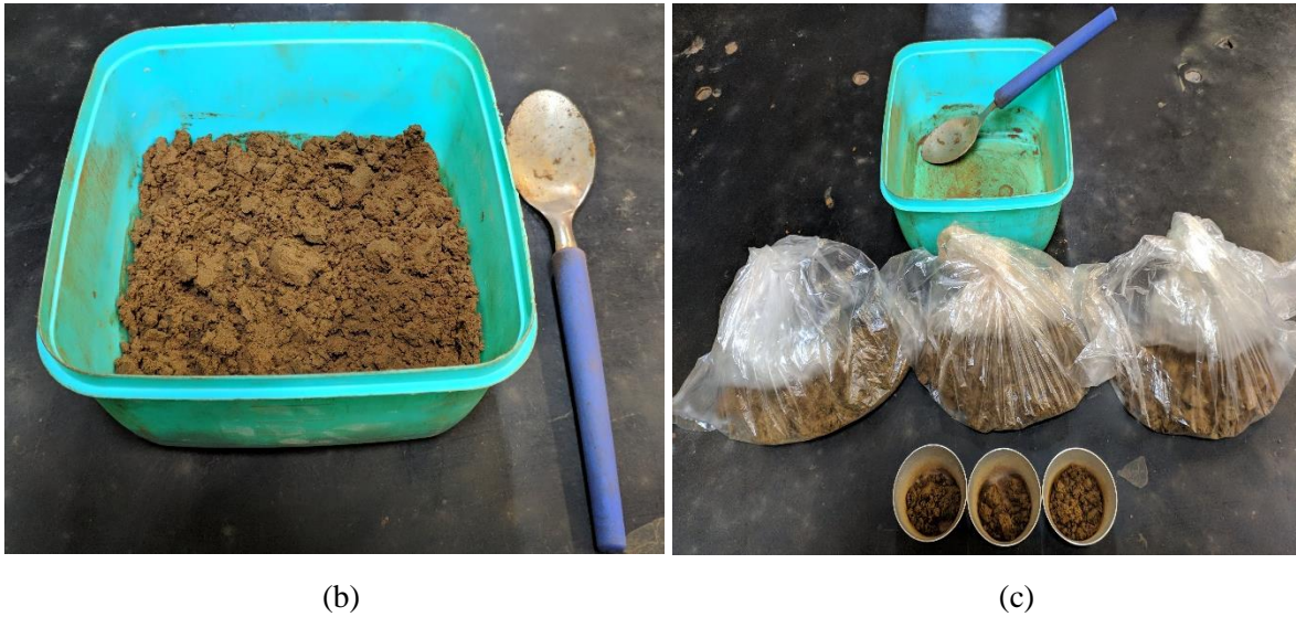
Figure 24: Samples' confection: a) soil, ordinary Portland cement and distilled water weighed according to the blends' dosage; b) materials homogenization and c) moisture content determination and specimens' layers division.
