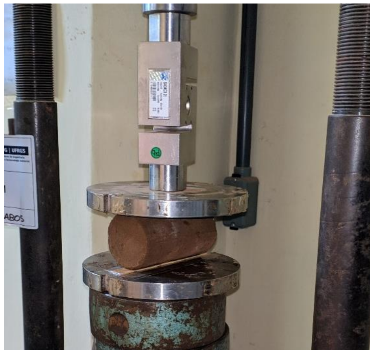
Figure 26: Unconfined splitting tensile strength test ongoing.
