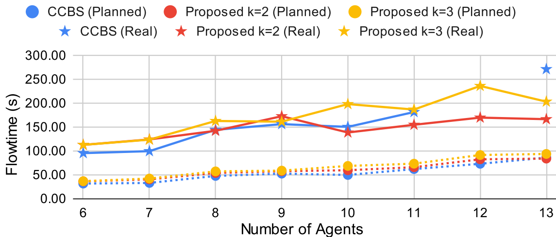
Figure 6.7 – Average flowtime values for the plans between all instances and for the flowtime measured after execution in Gazebo.
