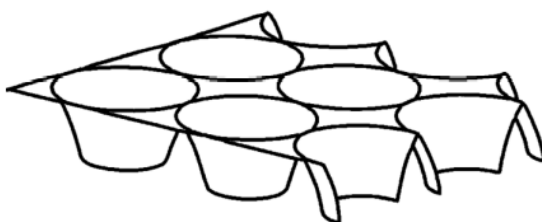
FIGURE 2.15. Two dimensional schematic representation of the muffin tin potential [46].
