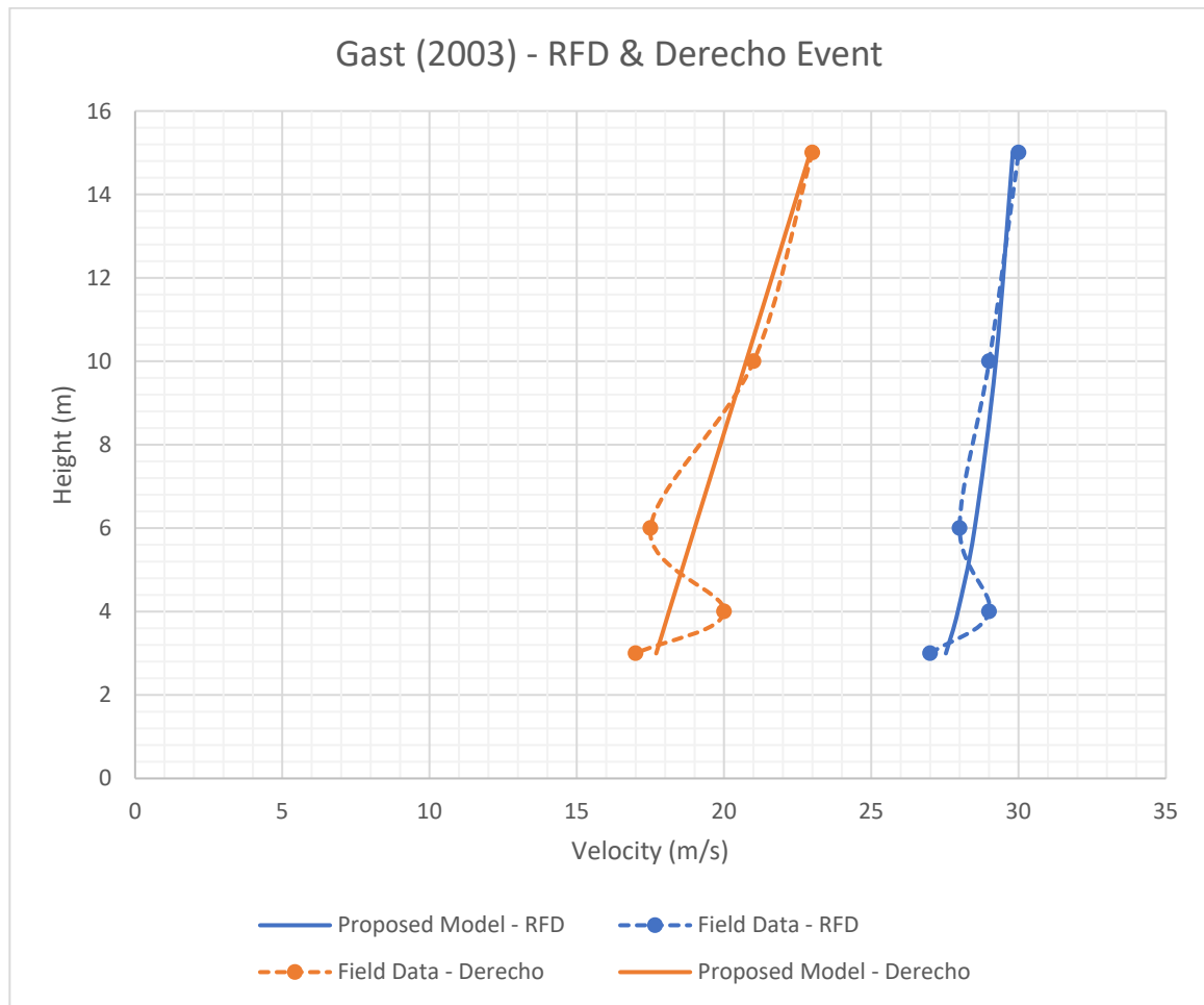
Figure 92. Proposed model (continuous blue line) and field data (dashed blue line) from vertical TS wind event extracted from Gast (2003) for RFD event and proposed model (continuous orange line) and field data (dashed orange line) from vertical TS wind event extracted from Gast (2003) for Derecho event. Source: Author.
