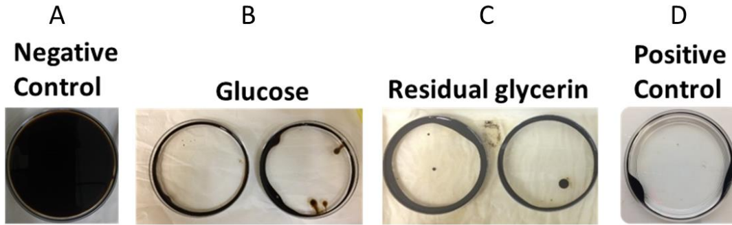
Figure 9. Oil spread assay. Positive results for both experimental conditions using glucose (B) and residual glycerin (C) as carbon source to produce BSFs. Negative control: MSM (A). Positive control: SDS 10% (D).
