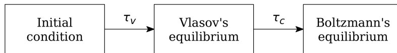
Figure 2 – Schematic description of the dynamical evolution of systems with LR interactions. First there is a violent relaxation at characteristic time \tau_v = O(1) , and then there is a collisional relaxation at characteristic time \tau_c = O(N^\zeta) .
