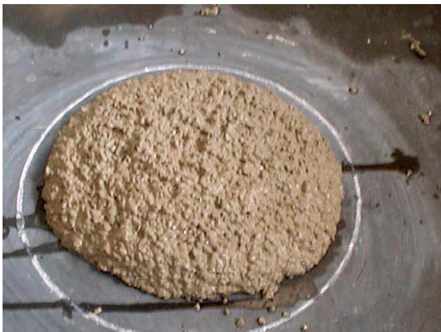
Figura 19: T50 Test ( Slump-flow Time )
