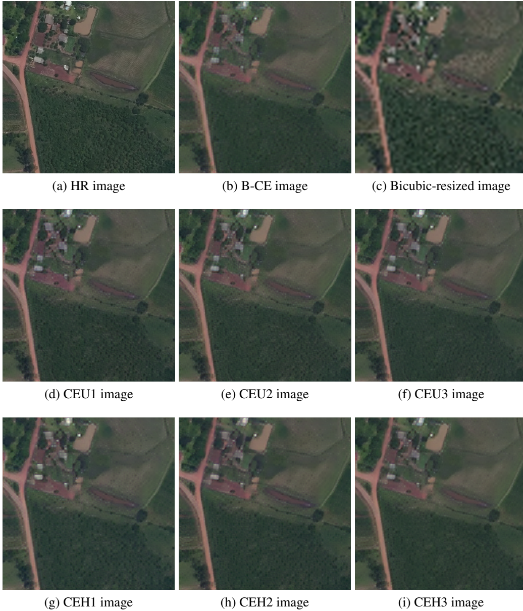
Figure A.1 – HR image, bicubic re-sampled image and inference results of Table 4.1 for the CGEO dataset using an ESRGAN-based SR module and UNet or HRNet segmentation networks.
