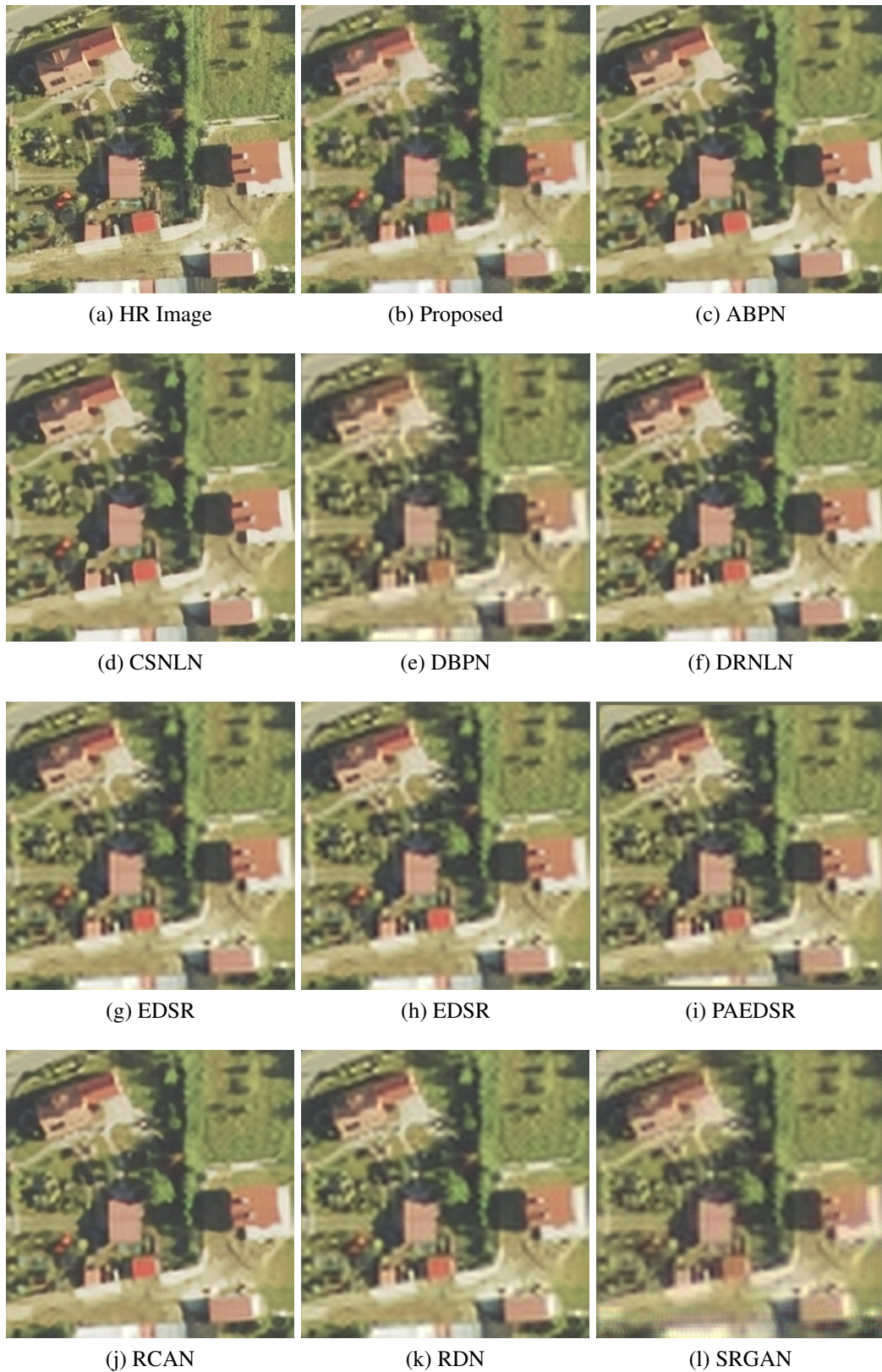
Figure C.2 – Comparison between proposed method and multiple SOTA super-resolution methodologies for x4 enhancement on the LCAI dataset.
