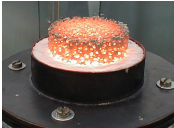
Figure 1.2 – SiC foam porous burner. Adapted: [Pereira et al., 2002]
