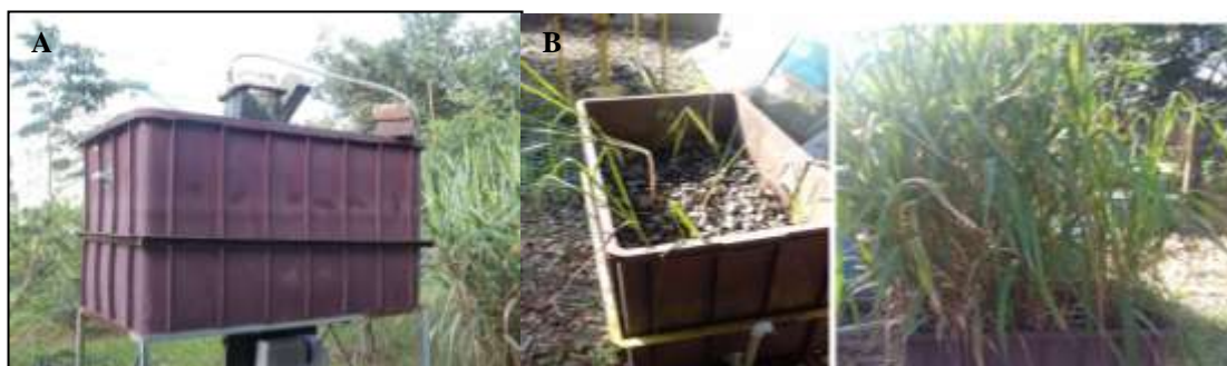
Figure 1: Schematic representation of the integrated wastewater treatment system. A: Microalgae unit. B: Vertical Sub superficial Constructed Wetlands (CW).
