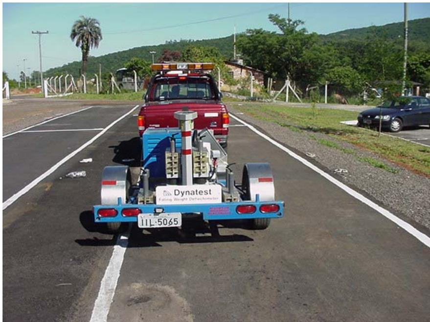
Figura 6.3: Falling Weight Deflectometer
