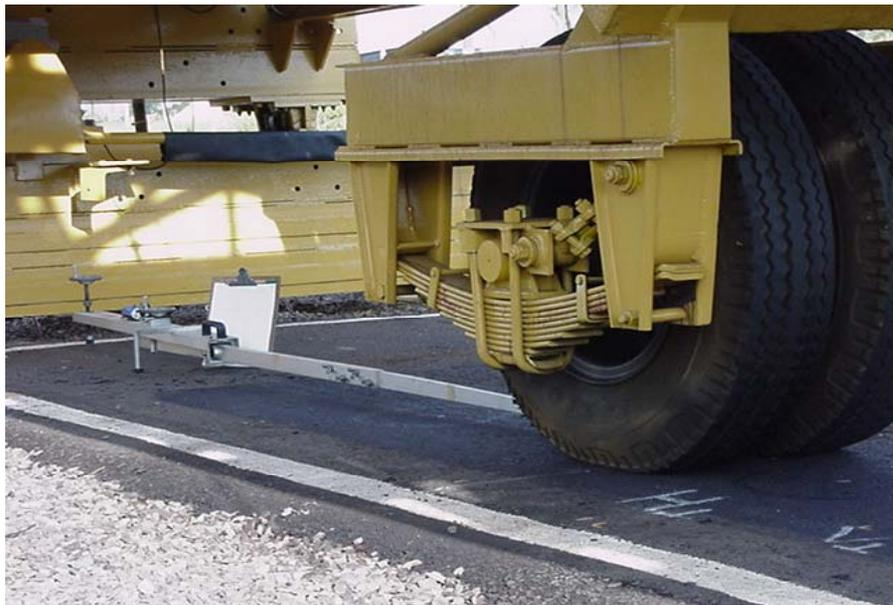
Figura 6.1: Viga Benkelman
