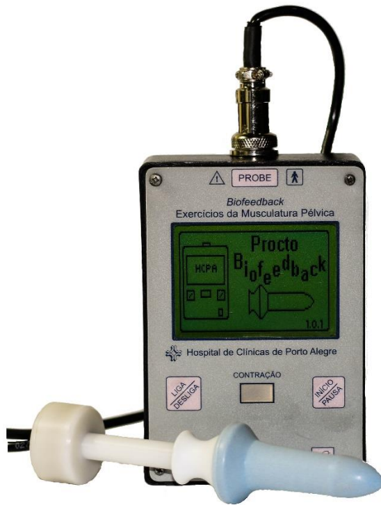
Figure 1 – Portable biofeedback device developed in the study
