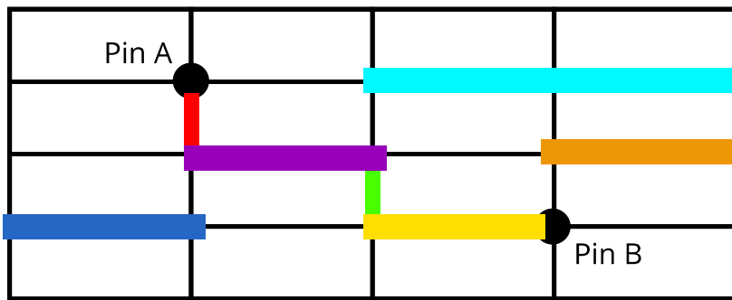
Figure 3.5: Example of a global connection routed by two partial assignments.
