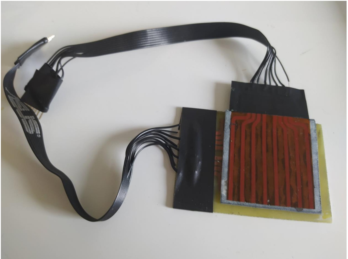
Figure 6.2: An 8x8 matrix device prototype based on PEDOT:PSS(diluted)@MS.
