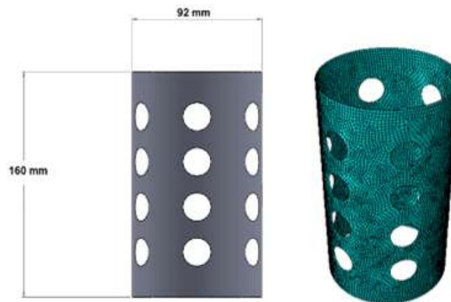
Figure 2. CHS mesh and geometric characteristics.
