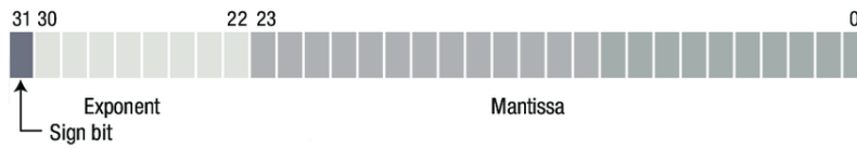
Figure 2.10: IEEE 754 single precision floating point decimal in binary.
