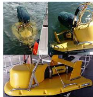
Figura 2. Chirp Sonar (0,5-12kHz) Edgetech 512-I
