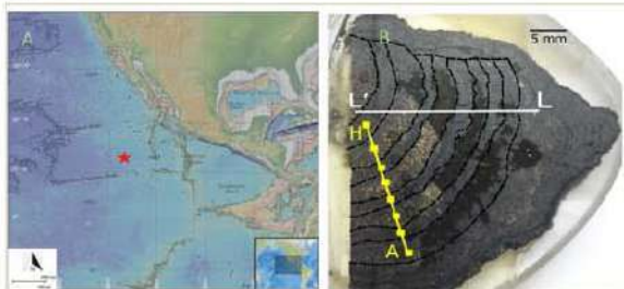
Fig.1: (A) Map showing Clarion Clipperton Zone, red star indicates the location of Fe-Mn nodule sample JC120-104B; (B) Ferromanganese nodule sample embedded in the resin. L-L' line shows the \mu -XRF (micro-X Ray Fluorescence) analysis profile, while A-H line shows the location of sub-samples (about 2mm cubes) collected for rock magnetic studies.
