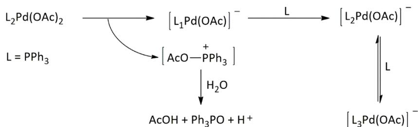
**Scheme 2.** Formation of active anionic  $\text{L}_n\text{Pd}(0)$  specie from  $\text{Pd}(\text{OAc})_2$  and  $\text{PPh}_3$ .
