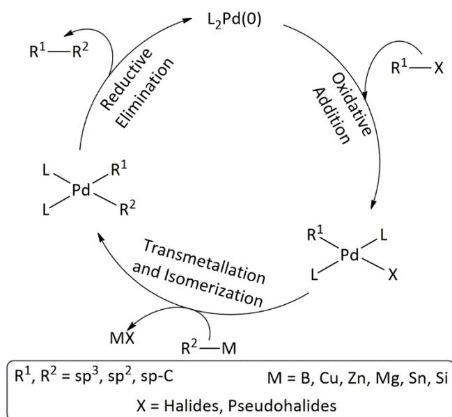
**Figure 6.** Proposed catalytic cycle for Pd-catalyzed cross coupling reactions.
