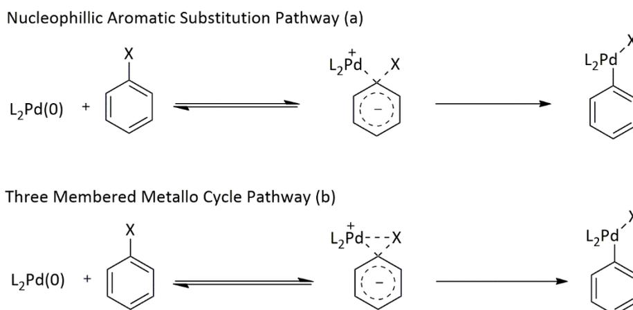
**Scheme 3.** Mechanistic pathways for oxidative addition.
