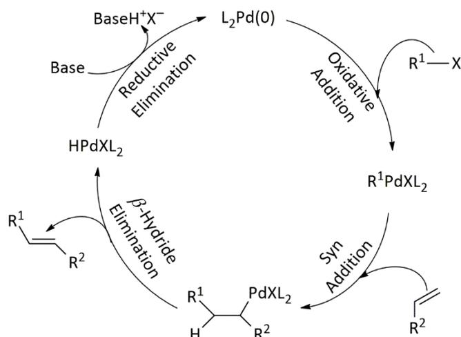
**Figure 7.** Mechanism of Heck reaction.
