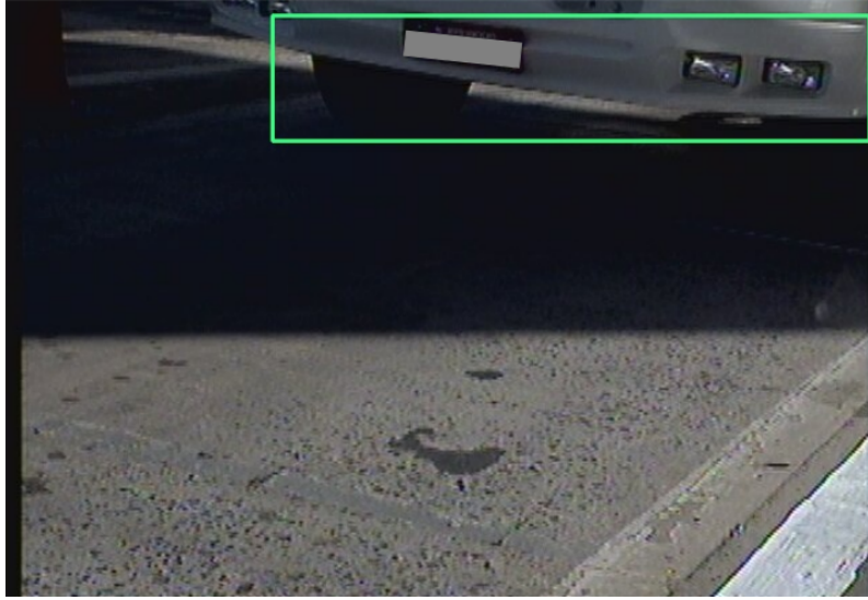
Figure 5.15: Bad LP detection example: applying WPOD-NET to the the vehicle bounding box (green rectangle) returns no LP. The LP is correctly detected when applying WPOD-NET to the full image.
