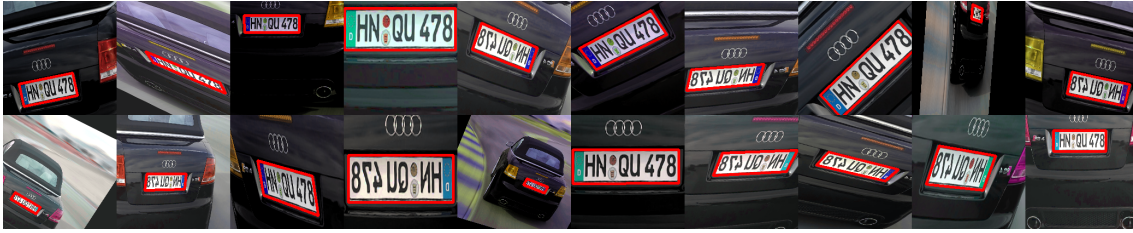
Figure 5.8: Different augmentations for the same sample. The red quadrilateral represents the transformed LP annotation.
