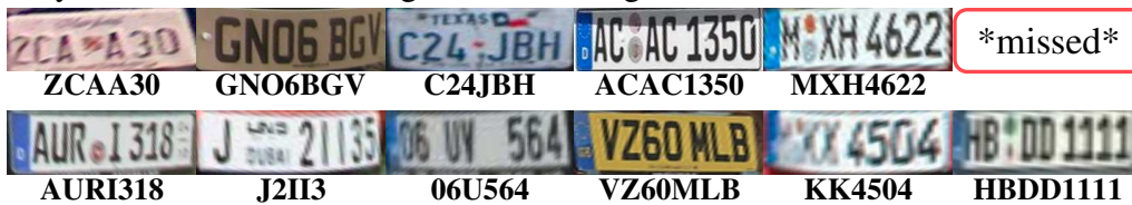
Figure 5.11: Detection results of WPOD-NET: unwarped LPs and final ALPR result produced by OCR-NET for the images shown in Figure 5.1.
