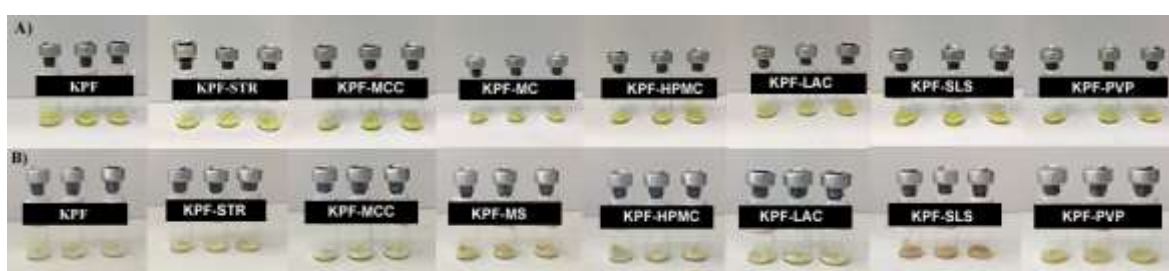
Figure 8. Results of qualitatively analysis to identify color changes of KPF and KPF-excipient mixtures before and after 3 weeks of storage. A) Samples analyzes immediately after preparation. B) Samples after 3 weeks of storage at 50 °C
