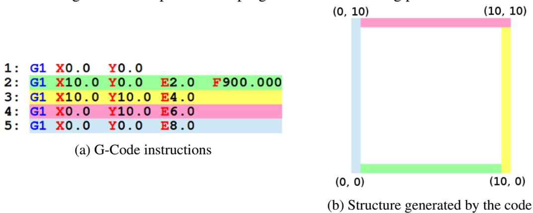
In the code depicted in (a), G1 is a move/extrusion instruction where: X and Y are the absolute coordinates where the movement will end; E is the amount of material to be extruded during the movement (cumulative); F is the rate the material will be fed to the extruder (thus, defines the movement speed). Each step is detailed below:
