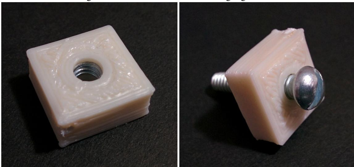
(a) 3D printed structure with nut partially visible
