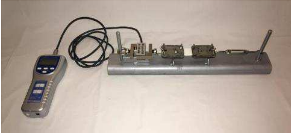
Fig. 2. System of clamps and screws used for graduated distension of the skin.
