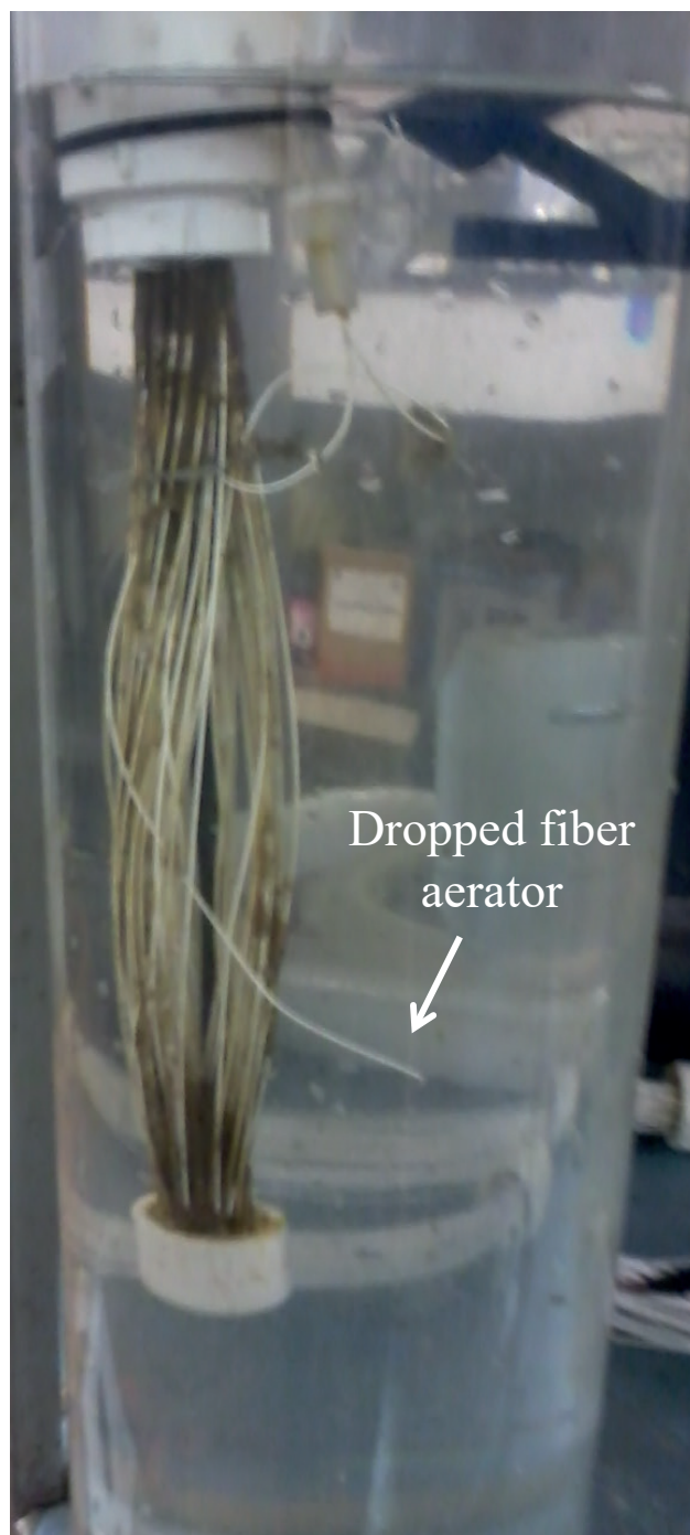
Figure 17. Photograph of the dropped fiber aerator for Mode 2 aeration and 5 L/min air flow rate.
