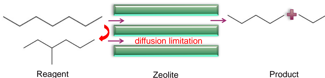
Figure 2-4 Schematic diffusion of reagents and products through the pores ZSM-5 zeolite (adapted from [29] ).
