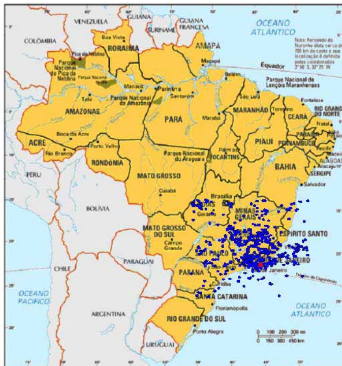
Figure 1: Distribution of epicenters of seismic events ( M_w \geq 1.5 ) recorded in the 54 years period between 1959 and 2013 within a 1200km square area in South-Eastern Brazilian SCR. The red triangle at (23.08° S, 44.45° W) shows the site of the Angra dos Reis NPP (CNAEA).
