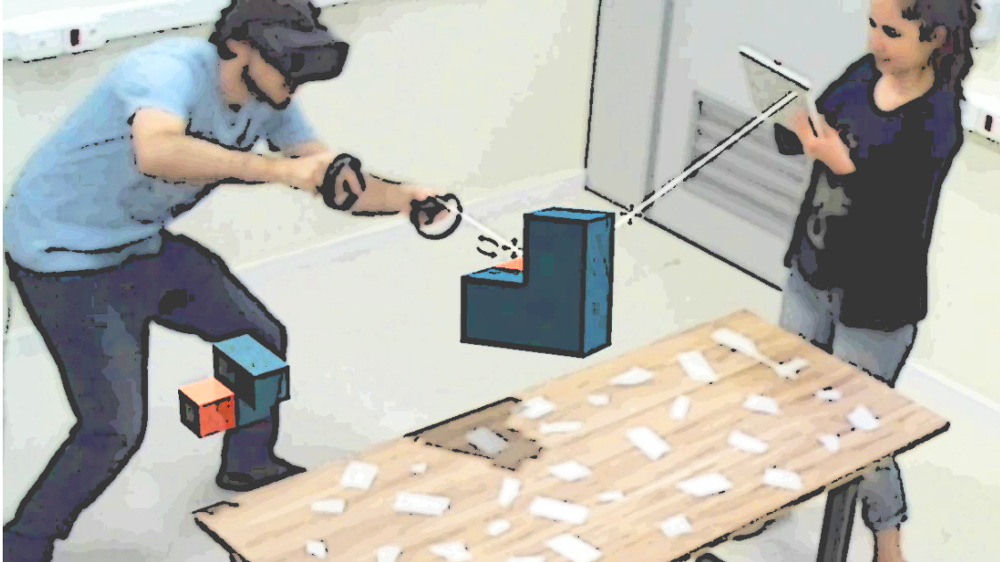
Figure 6.1: Asymmetric simultaneous interaction with mixed 3DUI techniques. Two co-located users are simultaneously interacting with a 3D object using different interfaces while sharing the same physical space.
