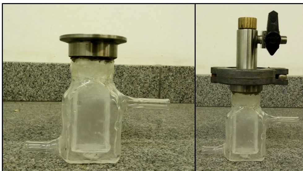
Figure 4.1.1 – Pictures of the quartz reactor used to perform the H 2 evolution photocatalytic activity measurements. The pictures present the quartz part and the stainless steel part used to seal up the reactor.
