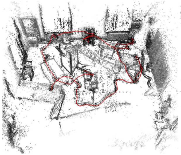
Figure 1.2: Visual 3D reconstruction
