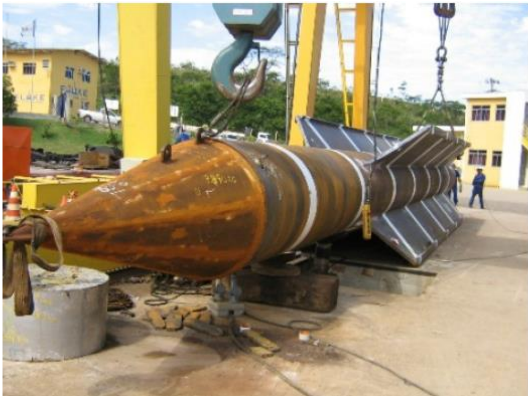
Figura 1.1 – Estaca torpedo (AGUIAR ET AL. , 2009)
