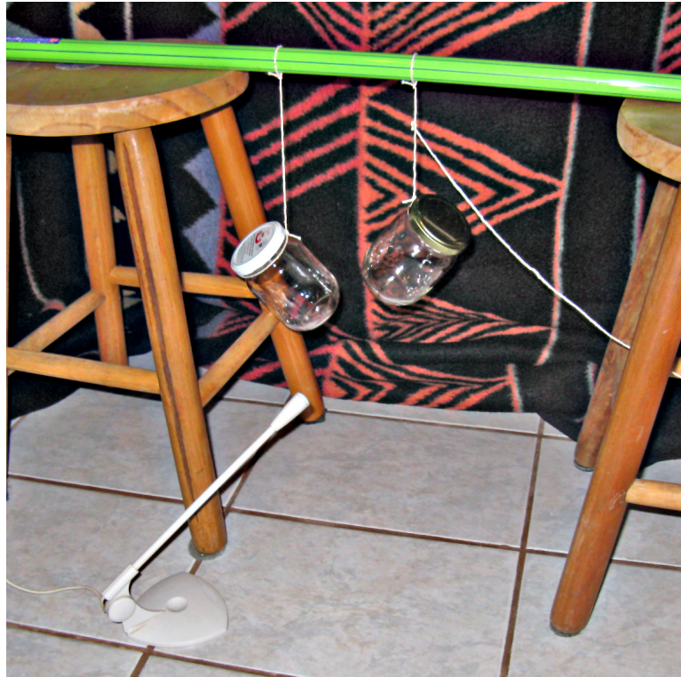
Figure 7.3: The setup environment for recording samples for the glass material. Two glass surfaces (the small glass jars) were suspended with threads, which were connected to a broomstick (at the top), which in turn was suspended on two small wooden stools. A microphone was placed directly below the jars, and a blanket surrounded the whole setup to help dampening some ambient noise. An additional thread was connected to one of the jars' thread (the right one) so that the jar could be swung from outside the recording area, allowing the blanket (on the background) to entirely cover these elements. Nonetheless, the sounds were recorded at a time of day where little noise was present, and several samples were recorded and later the best sample was selected. The same procedure was repeated for the sounds of plastic and wood materials, but then using plastic jars and wooden spherical objects instead.
