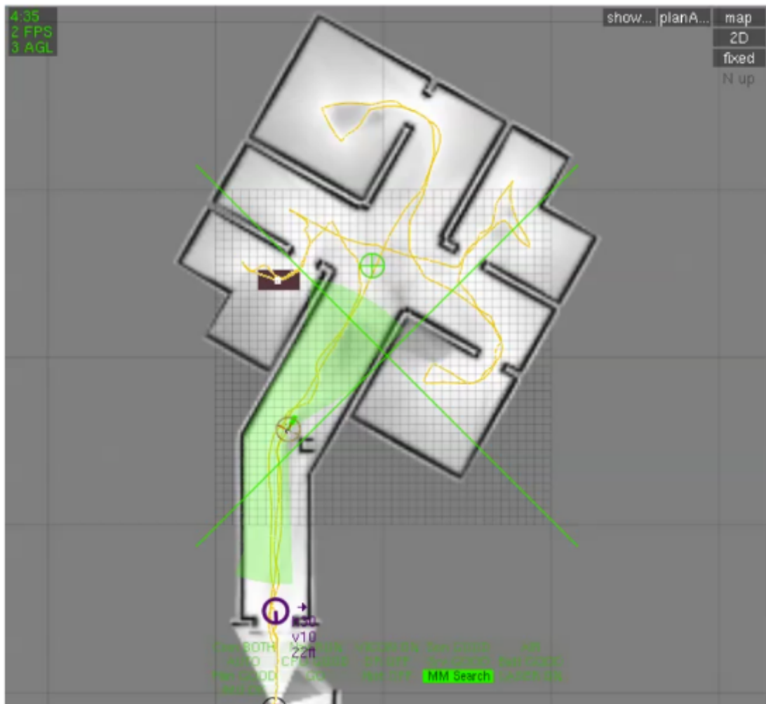
Figura 4: Result of the SLAM map and trajectory of the UAV while exploring a simulated indoor environment (MAGREE; JOHNSON, 2014).
