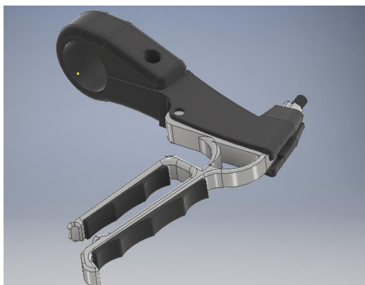
Figura 52: Modelo manete no Inventor Professional 2017
