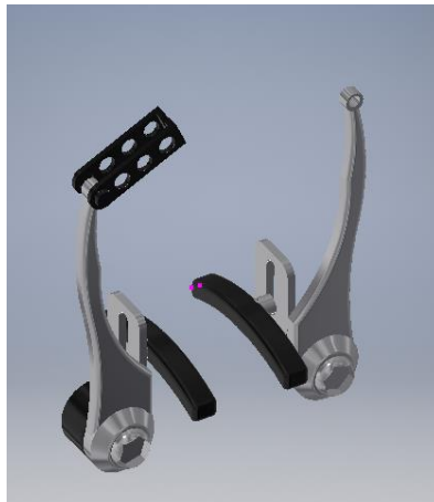
Figura 46: Modelo V-Brake Inventor Professional 2017
