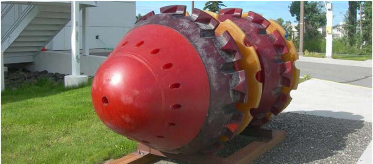
Figura 2.1 - Pipeline inspection Gage (PIG).
