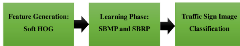
Figure 2.7: Block diagram of the SHOG + SBRP/SBMP classification process
