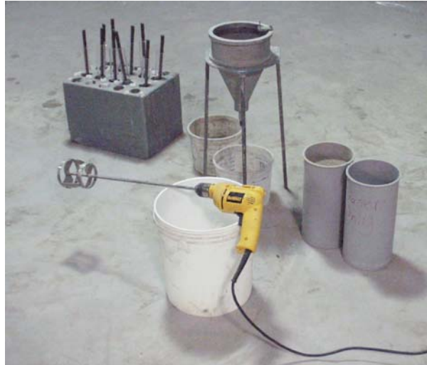
Figure 3.14 - Grout mixing and specimen casting ready to begin
