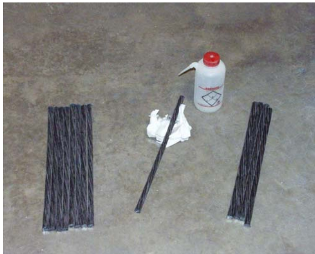
Figure 3.10 - Acetone was used to clean the strands prior to the casting step
