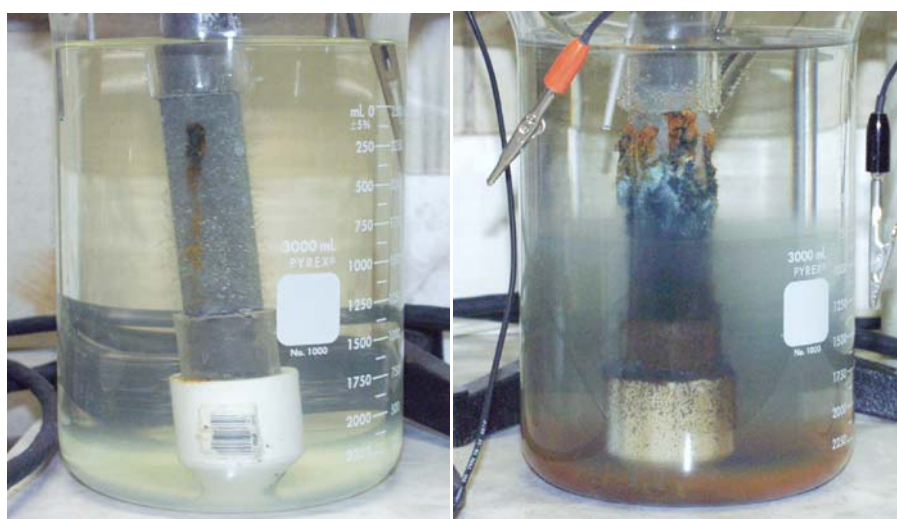
Figure 3.3 - Volume of corrosion products for low and high level of currents
