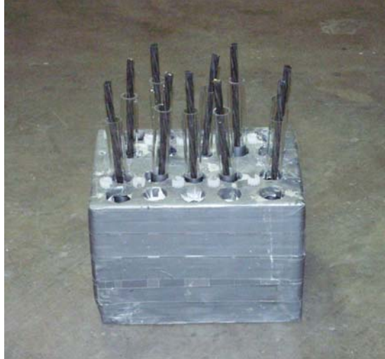
Figure 3.13 - Set of casings with placed strands ready for the casting procedure
