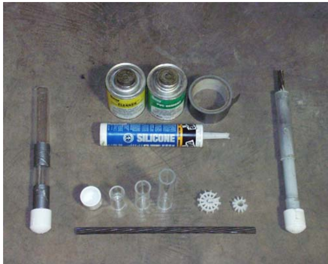
Figure 3.5 - The manufacture of an ACT specimen: in the middle, casing/specimen parts and products for caulking, gluing, and taping; on the left, an assembled casing; and, on the right, a completed specimen.
