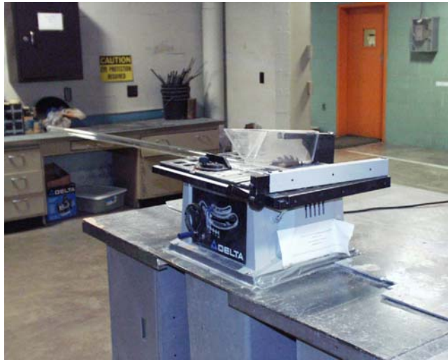
Figure 3.7- Clear tubing positioned in a bench saw for cutting of casing parts
