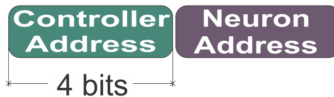
Figure 5.2: Cluster Level Packet, containing the Neuron and Cluster Addresses.
