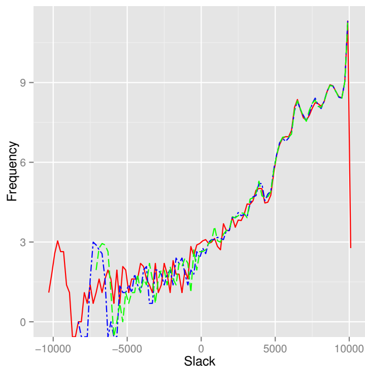
Figure 5.4: The slack histogram comparison for Superblue3. The red curve stands for the initial solution, the blue to the baseline flow and the green to the proposed flow.
