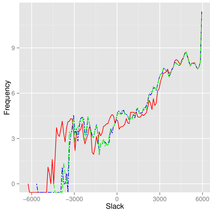
Figure 5.5: The slack histogram comparison for Superblue4. The red curve stands for the initial solution, the blue to the baseline flow and the green to the proposed flow.
