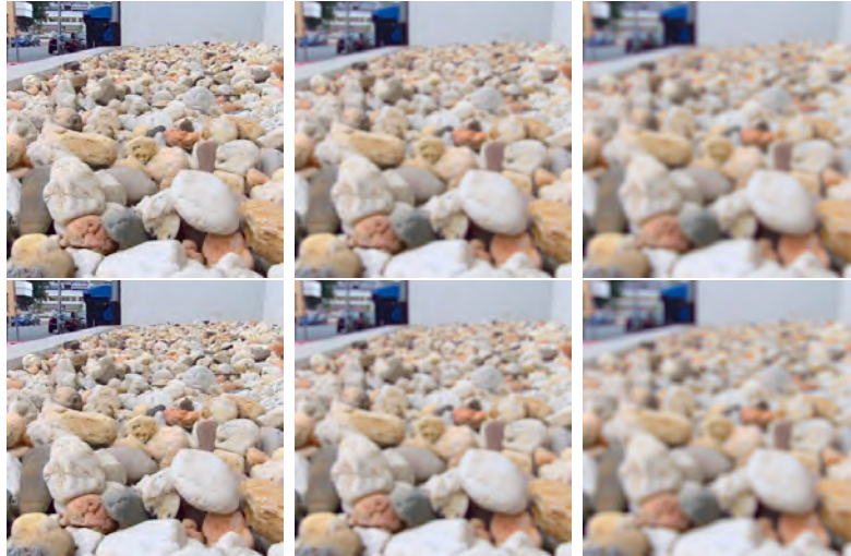
Figure 5.19: Artificially blurred natural image ( Image 19 ). First row using spatially-invariant Gaussian PSFs ( \sigma_b = 0.5 , \sigma_b = 1.65 and \sigma_b = 3 respectively) and second row corresponding disc blurry images ( r_b = 0.75 , r_b = 3 and r_b = 5.5 respectively). Source : (D'ANDRES et al., 2016)
