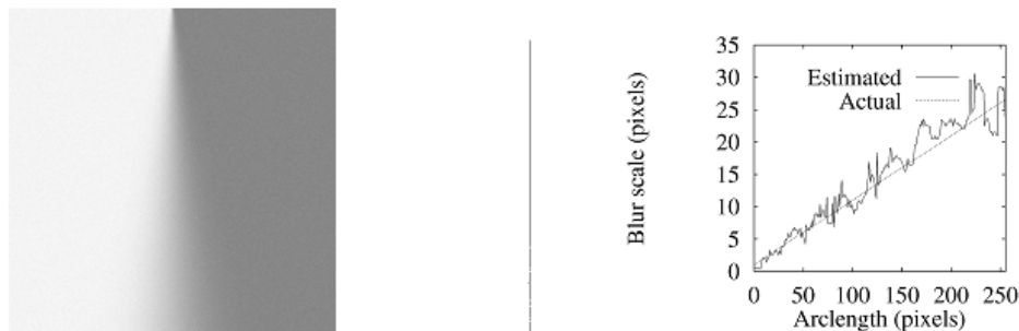
Figure 2.2: From left to right: the synthetic image, detected edge and estimated versus actual blur scale along the edge (ELDER; ZUCKER, 1998).
