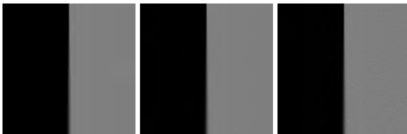
Figure 5.1: Artificially blurred edge stripe images with varying noise contaminations: from left to right no noise, \eta = 1.255 and \eta = 2.55
