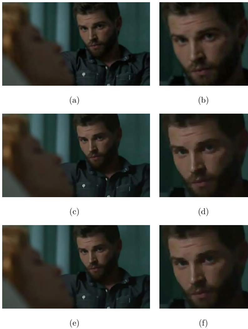
Figure 5.36: Video deblurring results for Video #1. Original image (a) and the selected patch (b), deblurring results using our defocus estimation method with (c) and without temporal coherence (e) and corresponding selected patches (d)-(f).
