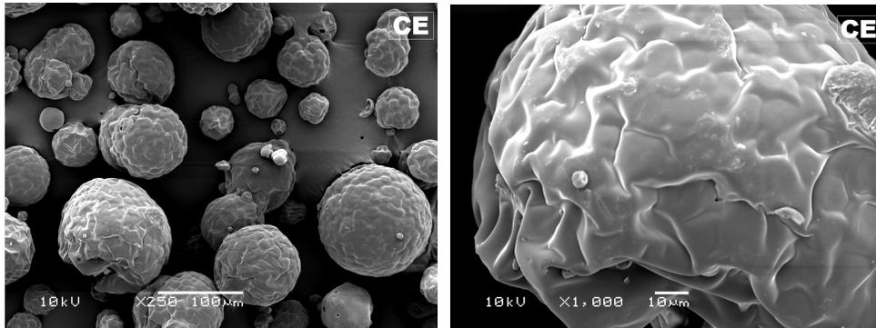
Figure 2: S.E.M. microphotographs of commercial extract (CE) with magnification of 250 and 1,000 times.
